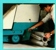
Main brush changes in minutes without tools. Many brush types assure optimum debris pickup in a variety of applications.
